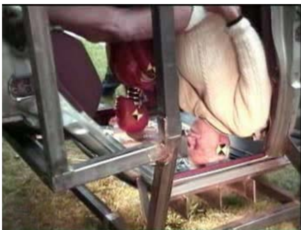
Figure 7a. Dummy (left) and human volunteer (right) in drop test fixture [19]
